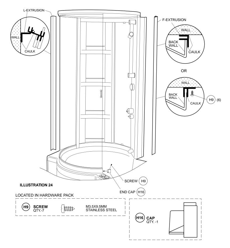
14. Install on the sides of the tower the aluminum extrusions provided. They may be sealed in place or secured with screws. Seal the end cap and place into the end of the lower track. Secure with self taping screw. (See Illustration 24.)
